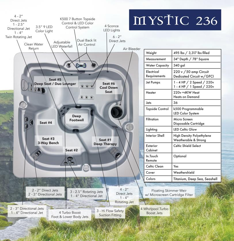
The Mystic 236 is our flagship therapeutic hot tub. The Turbo Boost Therapy System is powered by 2 - 4 HP jet pumps. The primary 2 speed jet pump will provide low or high speed therapy through 23 back jets. The second pump is focused on powering 8 - Turbo Boost Jets as well as 5 jets in the deep therapy seat.
